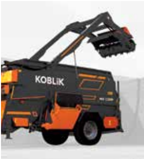
Loading the feed silo in the mixing hopper
