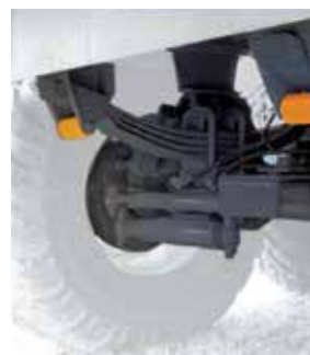
Hydraulic locking device of controlled axles for increased cross-country capability
