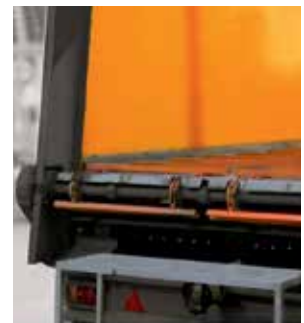
Dual drive of the unloading conveyor for smooth feeding without congestion
