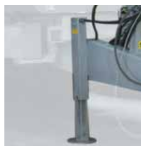
Hydraulic drawbar support for convenient parking
