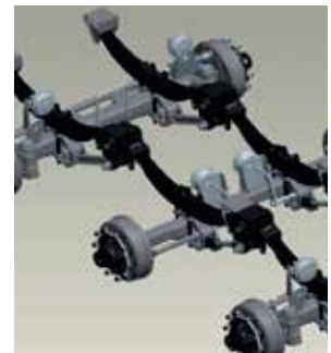
Balancing suspension of axles with parabolic springs
