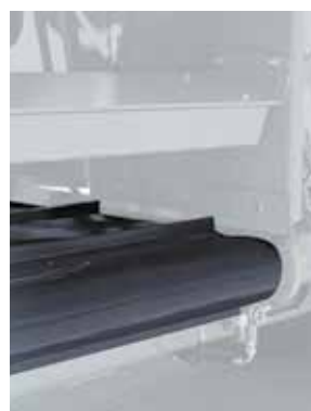
Reversible low-noise conveyor made of durable PVC tape
