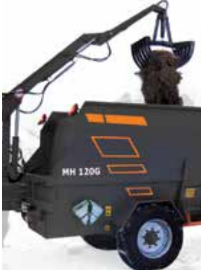
The angle of rotation of the grab is -240° without turning the machine
