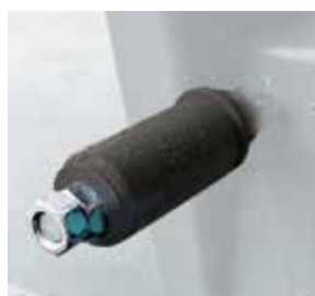
Mechanical chain tensioner of the unloading conveyor to protect against sagging and jerks
