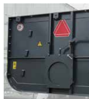
Hydraulic tailgate with automatic locking and an unloading window in the rear side for installing a screw loader
