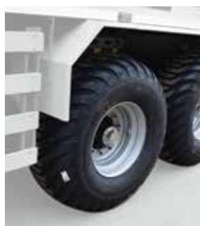
Tridem suspension with one or two pivoting/self-steering axles
