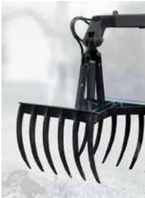
The maximum (and sufficient) boom reach is 3.2 m (loading height is 4 m)
