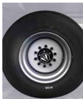
Large tires (235/75R17,5-305/70 R19.5) (reduced pressure and reduced frame loads)
