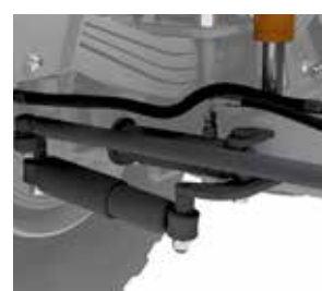
Hydraulic locking of steering axles for high cross-country ability
