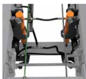
Stabilization of the body during unloading
