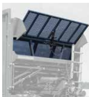
Semi-transparent front wall for full load control
