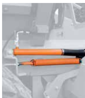
Hydraulic cylinders for conveyor drive control
