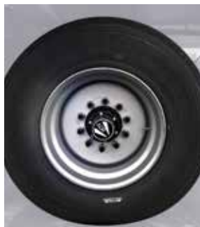
Large tires(385 / 55 R22,5 - 445 / 65 R22,5)(low ground pressure and reduced frame loads)
