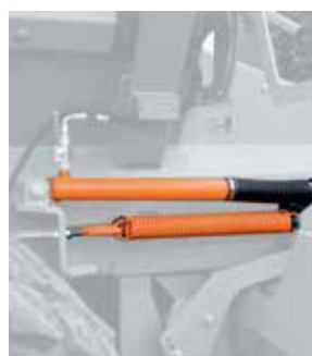
Hydraulic cylinders for conveyor drive control
