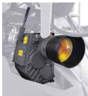
The gearbox reduces the load on the power take-off shaft
