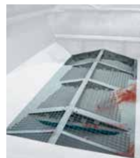
Stainless steel grate inside the hopper (protecting the product from litter and ensuring uniformity of filling)
