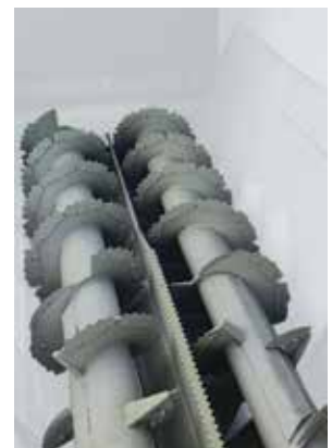
The diameter of the screws, taking into account the protrusion of the knives, is 540 mm with a dividing plate
