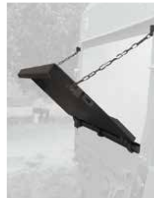
Opening lid on the back wall of the hopper
