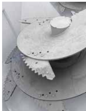
Two vertical cone-shaped augers
