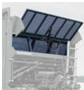
Semi-transparent front wall for full load control
