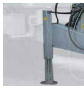
Hydraulic drawbar support for convenient parking
