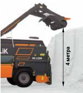
The lifting height of the milling cutter is up to 4 meters
