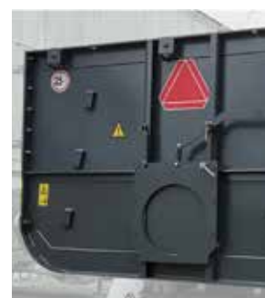
Hydraulic tailgate with seal and auto lock
