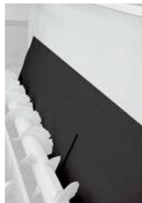
Possibility of execution of the bottom of the hopper with a thickness of 12 mm (long service life)
